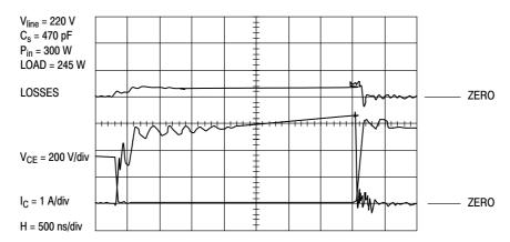
Figure 12. Losses in the Power MOSFET
