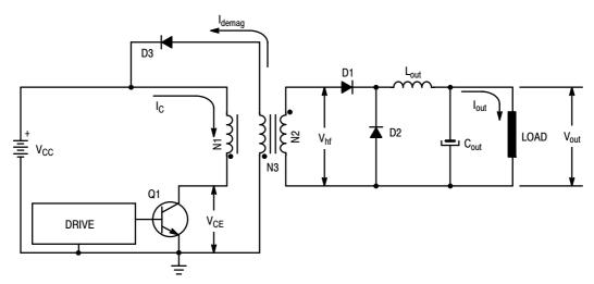
Figure 7. Basic Forward Converter Topology
