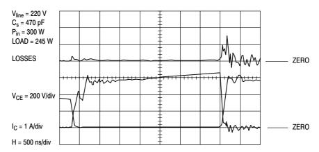
Figure 11. Losses in the Bipolar Transistor
