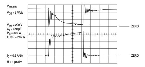
Figure 13. Dynamic  $V_{\text{CE(sat)}}$  of the Bipolar Transistor
