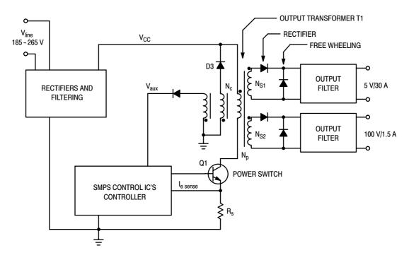
Figure 8. SWITCHMODE Power Supply Block Diagram
