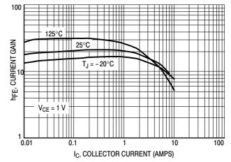
Figure 2. Typical Gain Curves for the Planar MJW18010
