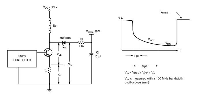
Figure 14. Dynamic On-voltage Test Circuit
