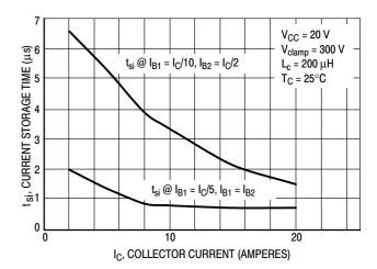
Figure 3. Collector Current Storage Time as a Function of I<sub>C</sub> and Base Bias (MJW18010)
