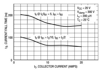
Figure 4. Collector Current Fall Time as a Function of I<sub>C</sub> and Base Bias (MJW18010)
