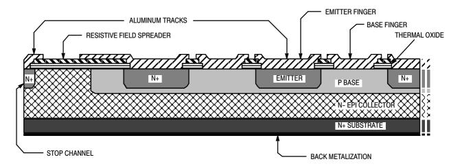
Figure 1. Cross Section of High-Voltage Planar Transistor
